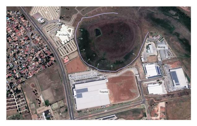
*Figure 53: Pan 1 showing the estimated location of the bioswale and expected points of stormwater discharge.*
