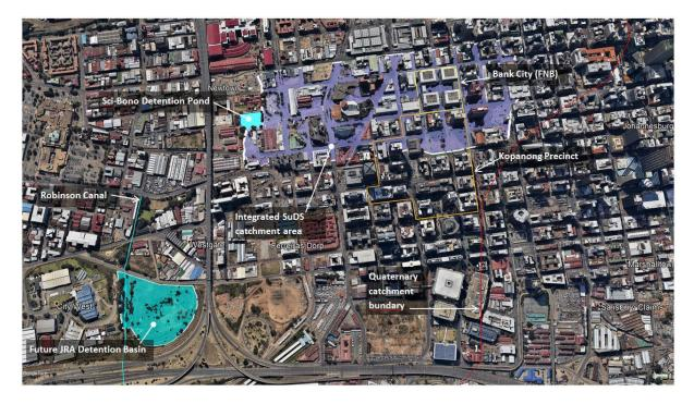
Figure 20: The CBD sub-catchment (blue shaded ground surface) used to analyse an integrated SuDS treatment train.
