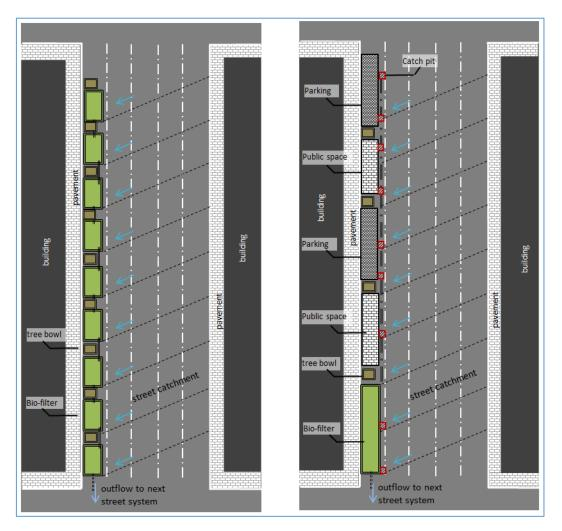
Figure 19: Schematic representation of street level interventions for the sample city block area; (left) Multiple bio-retention filters (each 7.5m<sup>2</sup>) interspersed with street features (trees, footpaths, benches, etc.), and (right) a single bio-retention filter (60m<sup>2</sup>) at the end of the street with the rest of the lane used for parking or public space
