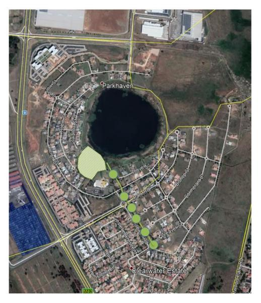
Figure 55: Preliminary SuDS concepts for Pan 2 showing a treatment train within the development space, and a possible wetland treatment system (hatched area) within the pan area
