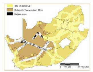
Figure 13: Map of South Africa indicating areas which are suitable for the installation of large concentrating solar power plants (Fluri, 2008)
