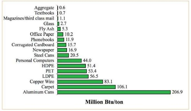
Figure 22: Energy Saving Potential per ton recycled
